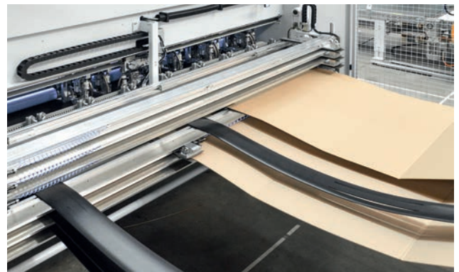
The endless carton changer is an automatic changing system for endless web widths with up to six compartments.
