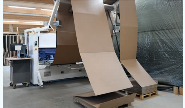
When using production lists , carton production is automated. Interruptions with individual cuts are possible without the last settings being "forgotten".
