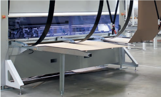
The combi-carton feeder enables the feeding of single sheets as well as the use of continuous cartons.
