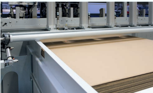
The single-sheet feeder enables the feeding of individual packaging sheets as well as the use of continuous cardboard without a reel.
